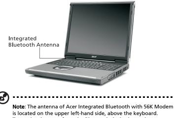
is located on the upper left-hand side, above the keyboard. Transmitted energy from the Bluetooth device is very low compared to other RF devices. Therefore, a 20 cm separation from the Bluetooth antenna is not required.
